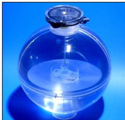
The Datawell stabilized platform sensor
